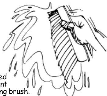
If your ground soil or your wall are damp or are subject to moisture intrusion, it is possible that efflorescence will reappear.
