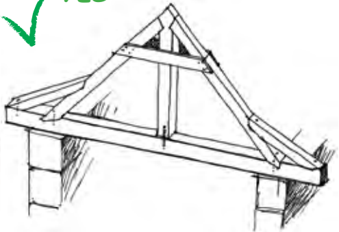
Building with solid timber : GOOD
