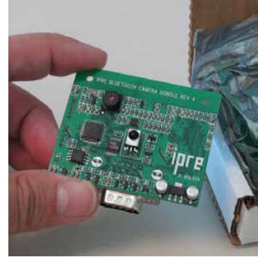
The Fluke Dongle adds Bluetooth and other capabilities to the Scribbler.
