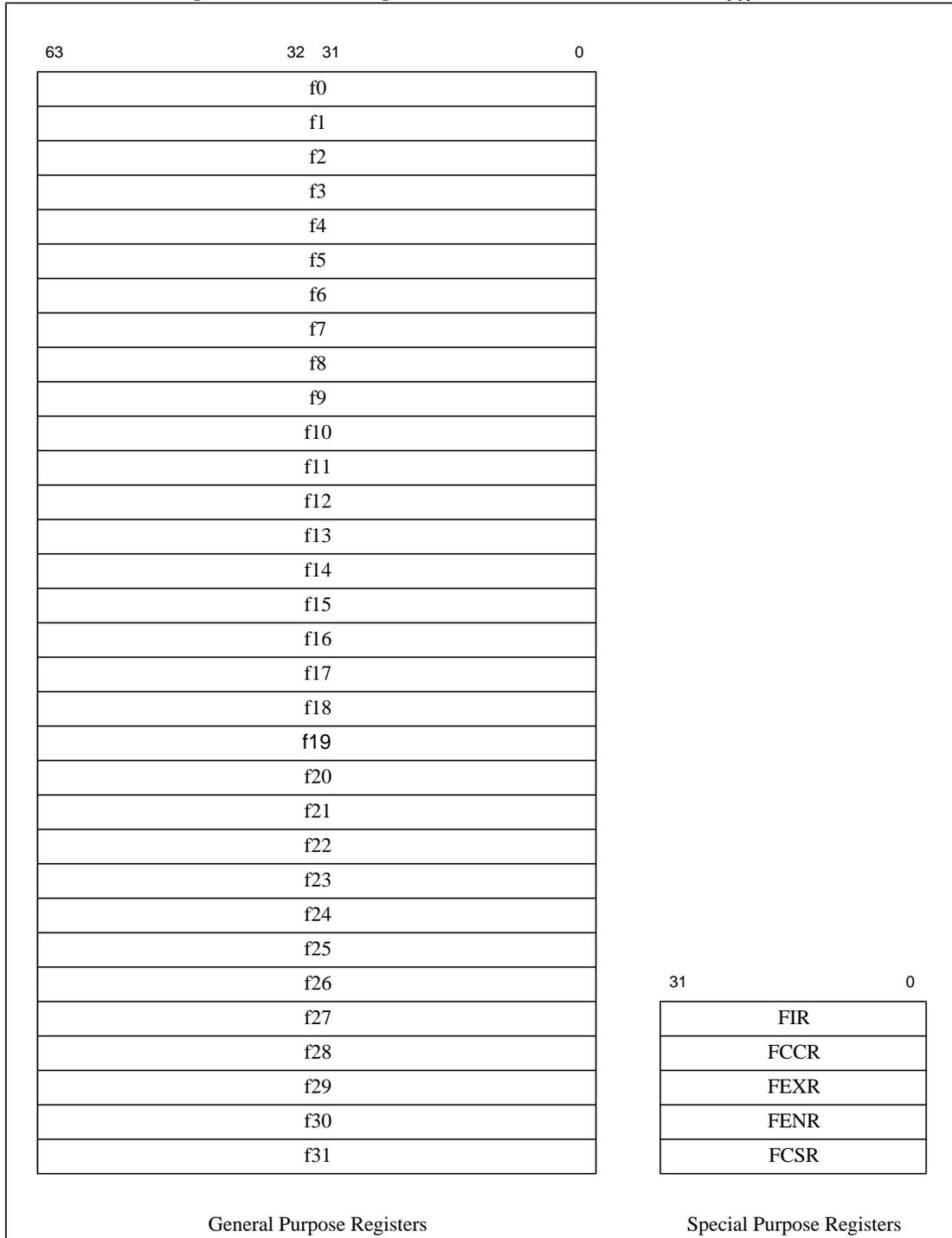
Figure 2-9 FPU Registers for a 64-bit FPU if Status<sub>FR</sub> is 0
