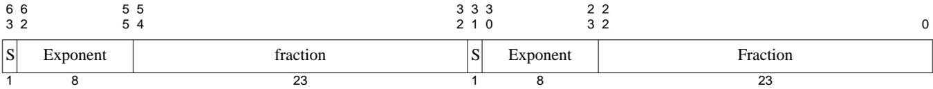
Values are encoded in the specified format by using unbiased exponent, fraction, and sign values listed in Table 5.31. The high-order bit of the *Fraction* field, identified as  $b_1$ , is also important for NaNs.
