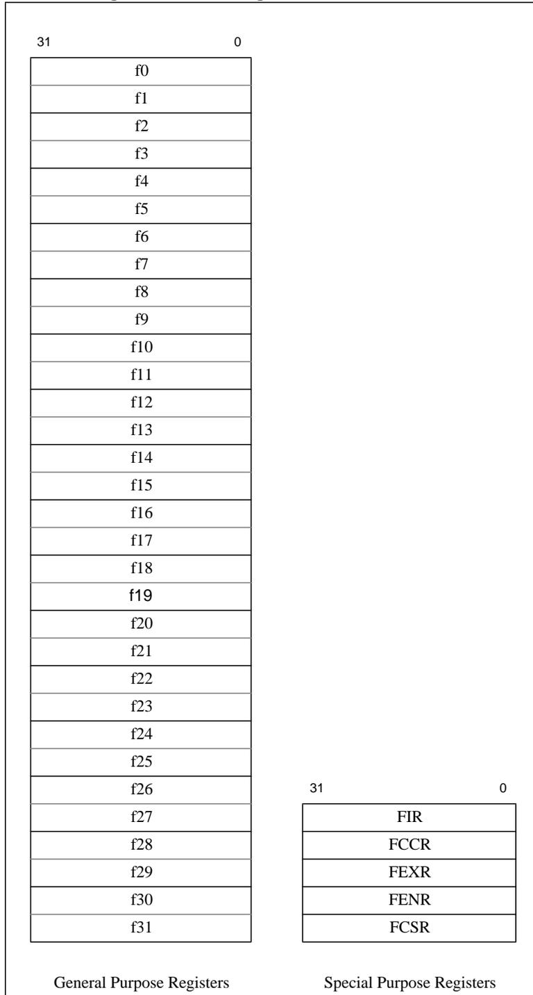
Figure 2-8 FPU Registers for a 64-bit FPU if Status<sub>FR</sub> is 1
