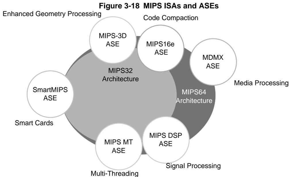
The MIPS32 Architecture is a strict subset of the MIPS64 Architecture. ASEs are applicable to one or both of the base architectures as dictated by market need and the requirements placed on the base architecture by the ASE definition.
