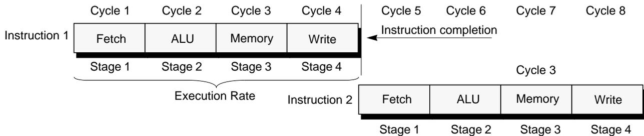
In the example shown in Figure 2-2, each stage takes one processor clock cycle to complete. Thus it takes four clock cycles (ignoring delays or stalls) for the instruction to complete. In this example, the **execution rate** of the pipeline is one instruction every four clock cycles. Conversely, because only a single execution can be fetched before completion, only one stage is active at any time.
