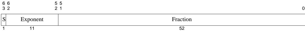
Figure 5-24 Paired Single Floating Point Format (PS)
