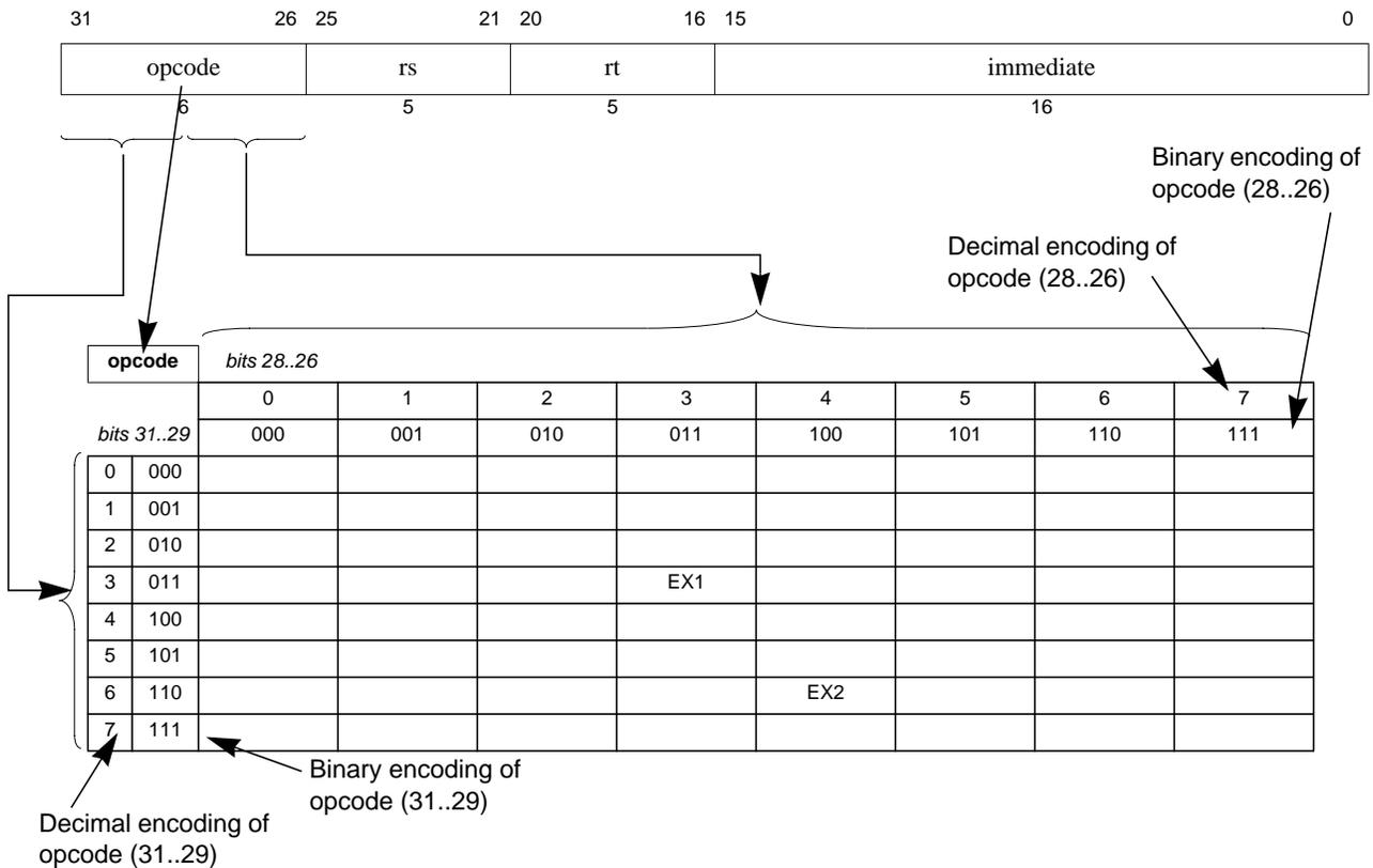
Tables A.60 through A.78 describe the encoding used for the MIPS32 ISA. Table A.59 describes the meaning of the symbols used in the tables.
