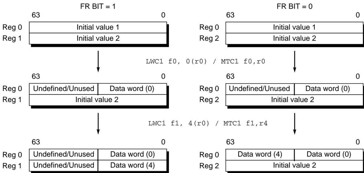
**Figure 5-28 FPU Doubleword Load and Move-to Operations**
